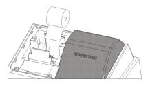
• Insert the paper roll (57 mm width) for the receipt in the paper holder. Bend the roll support a little to the left. The end of the paper roll must be at the bottom.
